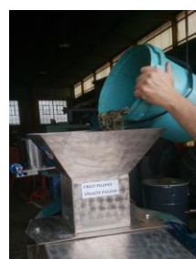
Fruit pulper separating seed from the pulp
